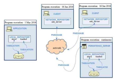
Figure 3.1 – Application and client/server dataflow
