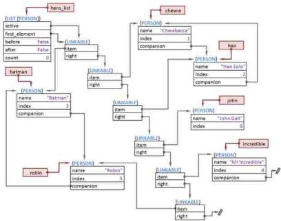
Figure 1.4 – Run-time object structure
